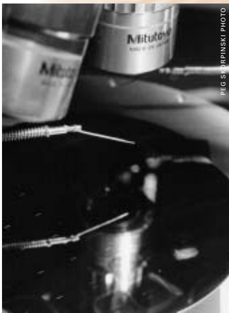
Probe stations, such as this one in the Device Characterization Lab, measure devices as small as a single transistor.
