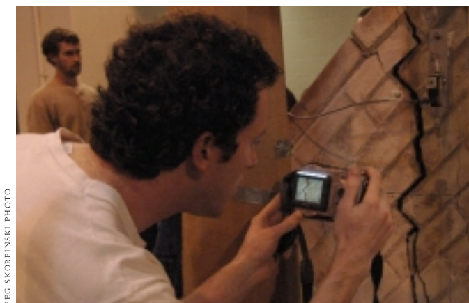
CEE graduate student Reid Senescu monitors the width and extent of cracks that finally caused the masonry specimen to fail. The shear tests were funded by the NSF, the Hellman Family Faculty Fund, and Sika Corporation.
