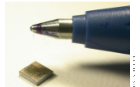
The wireless mote integrates radio frequency communication onto a sensor processing chip just 5 square mm in size.
