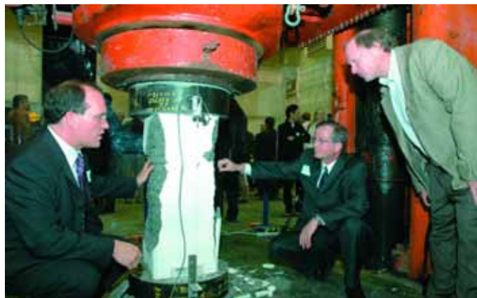
The massive Universal Testing Machine subjected a concrete column specimen to 2 million pounds of load in an earthquake simulation at the NEES opening. Inspecting the damage are (from left) Berkeley’s Bozidar Stojadinovic and Jack Moehle, and Mark Coles of the NSF.
