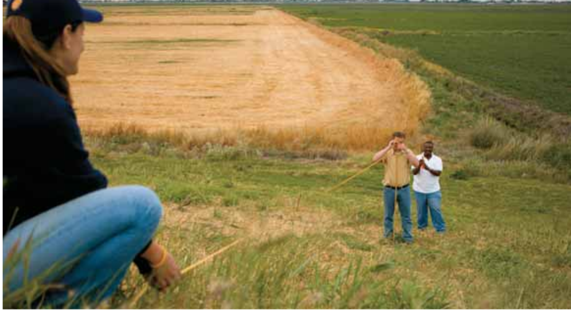
Adda Athanasopoulos (left), Rune Storesund (center) and Kofi Inkabi use tape and hand level methods to document the levee's geometry. Like New Orleans, the Delta levees are slowly subsiding, requiring constant maintenance to keep them at their specified level of protection.
