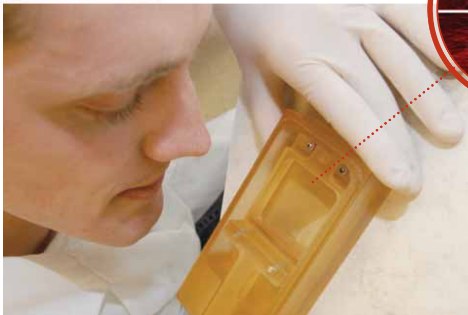
Bioengineering graduate student Kyle Kurpinski holds the device he developed for "stretching" stem cells, training them to take on the characteristics of the smooth muscle cells found in vascular tissue. Fibers in cells stretched on grooved membranes (inset) were encouraged to differentiate even further.
