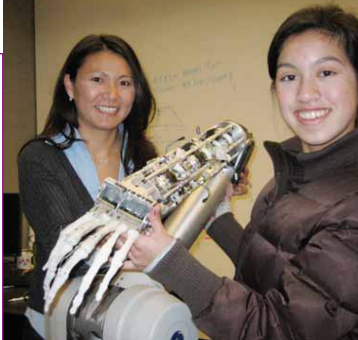
Yoky Matsuoka (left) and 8th-grader Olivia Pineda demonstrate Matsuoka's anatomically correct robotic hand, designed to integrate directly with the human body and brain.
