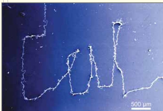
Liwei Lin and colleagues used near-field electrospinning to spell "Cal," demonstrating that nanofibers could be deposited in a controlled manner rather than the tangled mass resulting from earlier methods. The technique has potential for producing specialized wound dressings and chemical detectors.
