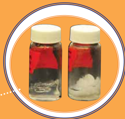
When the injectable hydrogel (left) reaches a temperature above 34 degrees Celsius, it undergoes a phase transformation, becoming stiffer and opaque (right).
